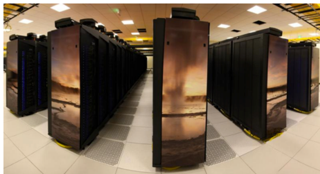
NCAR's Yellowstone is a 1.5-petaflops high-performance computing system with 72,288 processor cores.
