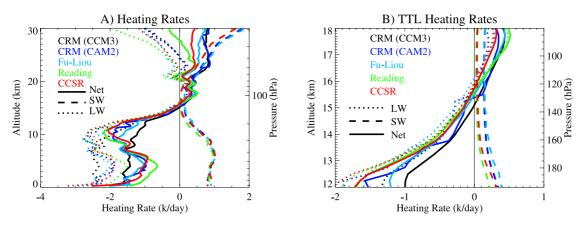
**Figure 4.** Profiles of Net (solid), Shortwave (SW- dashed) and Longwave or Infrared radiation (LW- dotted) from 5 different models. (a) Heating rates (in K day<sup>-1</sup>) from 0–30 km. (b) Heating rates (in K day<sup>-1</sup>) in the Tropical Tropopause Layer from 12–18 km. Individual models colored: NCAR CRM (CCM3 version) black, NCAR CRM (CAM2 version) dark blue, Fu-Liou light blue, Reading green and CCSR red.
