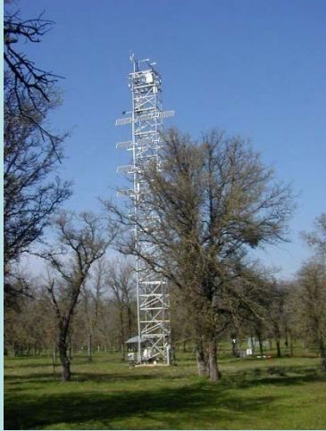
Eddy covariance flux tower (courtesy Dennis Baldocchi)
