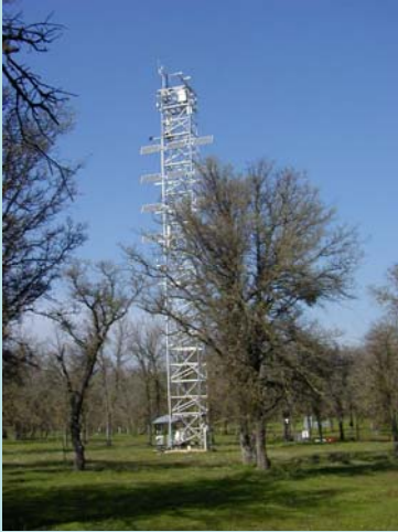
Eddy covariance flux tower (courtesy Dennis Baldocchi)
