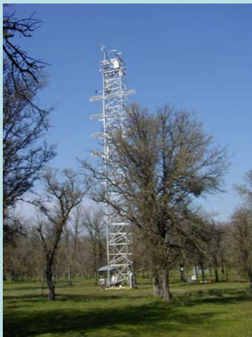
Eddy covariance flux tower (courtesy Dennis Baldocchi)
