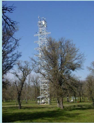
Eddy covariance flux tower (courtesy Dennis Baldocchi)
