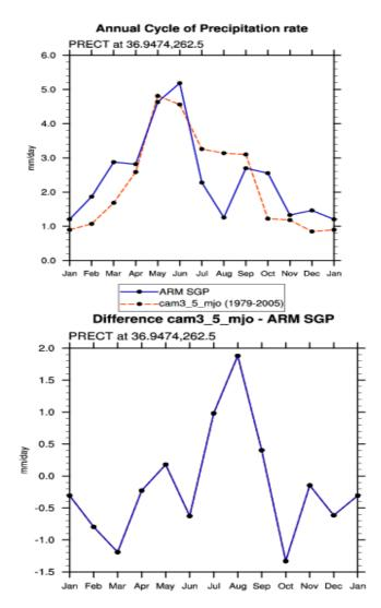
Figure 3. Mean annual cycle of precipitation from an AMIP run of the CCSM4 atmosphere component and observations in the Southern Great Plains of the USA.
