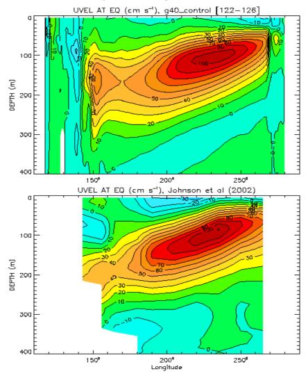
Figure 4. Comparison of zonal velocity along the equator in the upper Pacific Ocean between the ocean component of the CCSM4 and the observations in [30].
