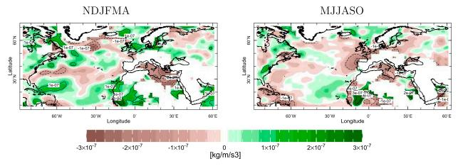
FIG. 9. The multimodel mean change from 1979–2005 to 2021–40 in the low-level (925 mb) mean convergence for the (left) winter and (right) summer half years. Negative changes imply increased low-level divergence. Units are  $s^{-1}$ .
