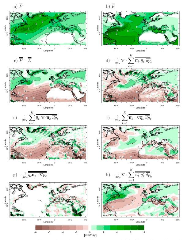
FIG. 1. The November–April half-year climatological moisture budget from ERA-Interim: (a) P, (b) E, and (c) P - E. (d) The moisture convergence by the mean flow and its components due to (e) mass divergence and (f) advection. (h) The transient eddy moisture convergence and (g) the surface term.
