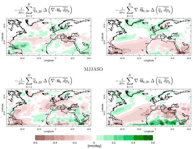
FIG. 8. The mean circulation (left) dynamical and (right) thermodynamical contributions to the change in the mean flow moisture convergence for the CMIP5 multimodel mean for the (top) winter half year and (bottom) summer half year. Units are millimeters per day.
